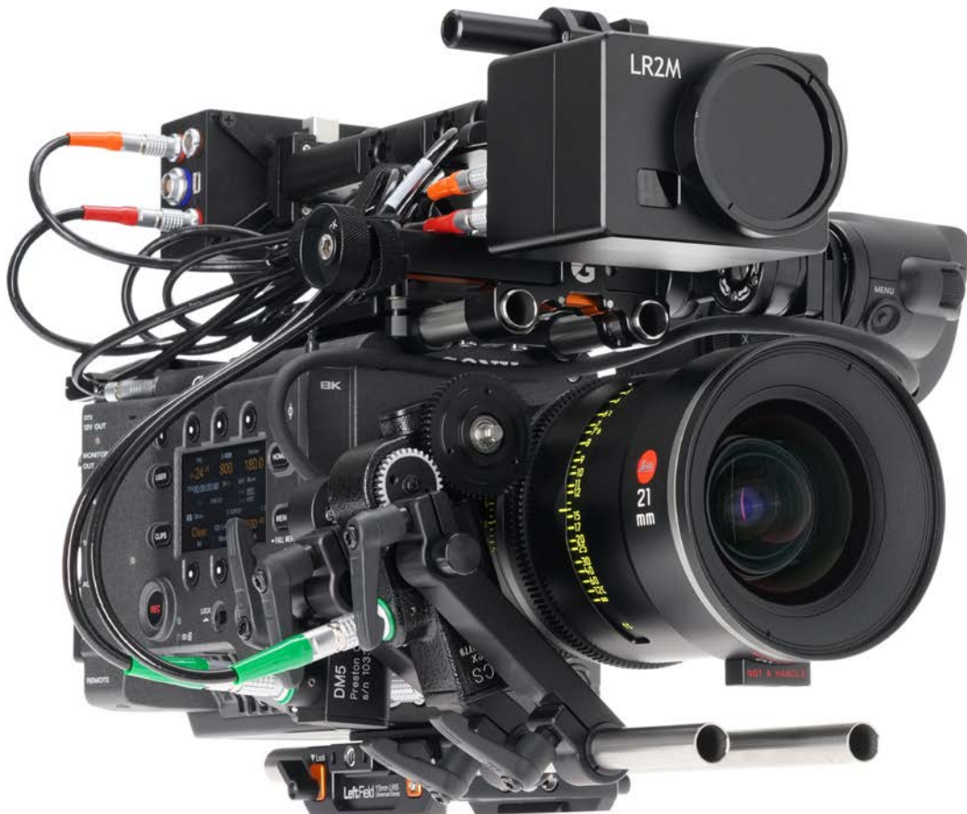
Sony VENICE 2 8K with Preston Light Ranger 2, Bright Tangerine Misfit Kick and Expert Kit, Leitz Prime.
